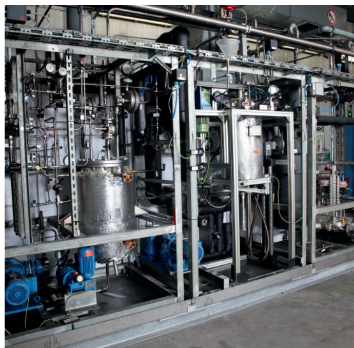
Test plant with stirred reactor for reactions in the gas/liquid phase
