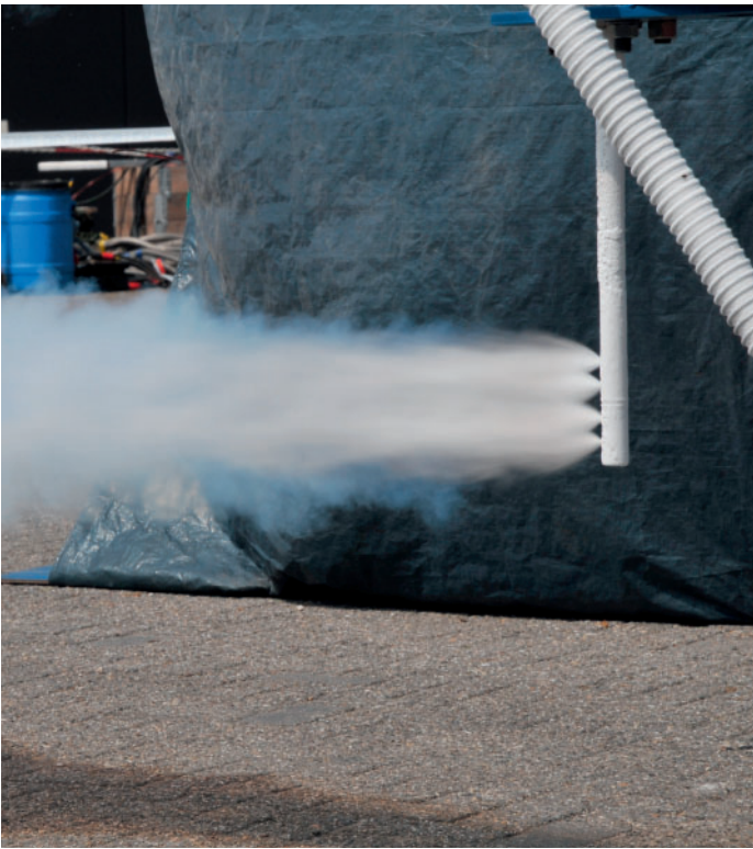
Injection of liquid nitrogen according to the CATCOOL™ process – a demonstration trial
