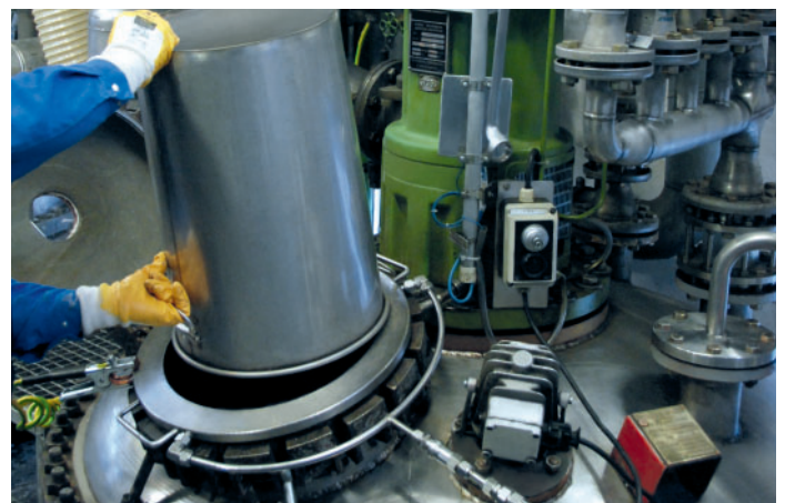
N2LOCK® inert-gas lock for safe manual filling of bulk material
